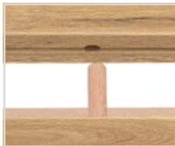
Solid dowel joint
